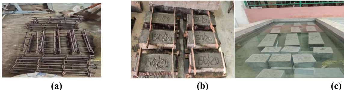
Fig.2 (a) Reinforcement cages (b) casting in wooden moulds (c) curing under water
